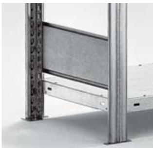
The frame support is a galvanized T-profile. With slots at increments of 25 mm, any desired arrangement of the shelving levels can be achieved. The shelving frames can be combined into the desired product using cross beams, closed side walls or mesh walls.
