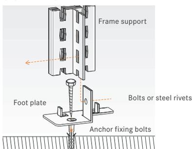
Foot plate (steel foot) bolted or riveted
