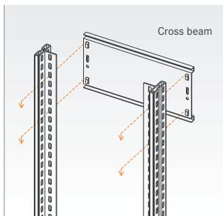
If the shelving height exceeds five times the shelving depth, the shelving must be protected against tipping – e.g. using wall fixings (in solid walls with extraction value of 150 N - corresponds to around 15 kg), by bolting together (cross bracing), or through bolts in the floor.
