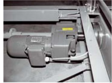
All electric drives are directly connected to the carriage drive shaft. The drive shaft is attached to the driving wheels by a flange coupling.
